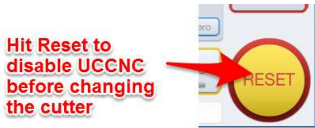
Figure 12: Reset to disable spindle relay
