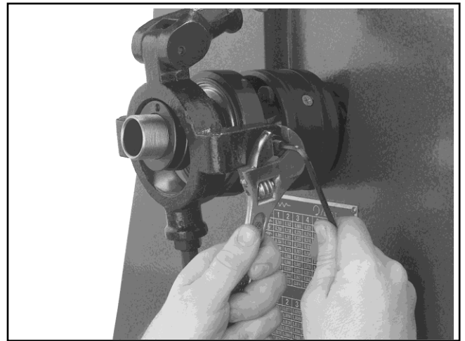
Figure 10. Tightening yoke setscrews.
