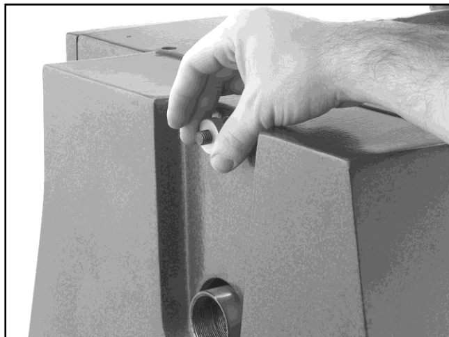
Figure 1. Lathe cover removal.
