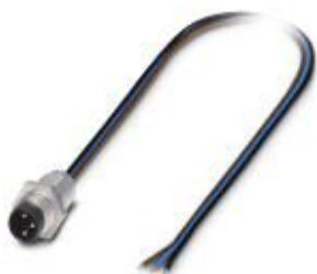
Flush-type connector, 3-position, Plug, straight, M8, Front mounting, M8 x 0.5, Individual wires, cable length: 0.5 m, 0.25 mm², PVC litz wire
